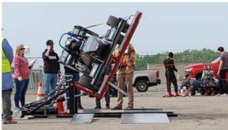
Fig. 3. PBR 23 on the tilt test
