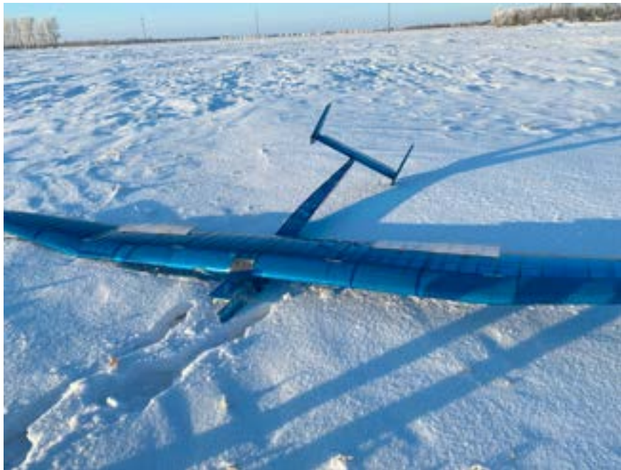
Crash-landed prototype plane after flight test at Steinbach South airport
